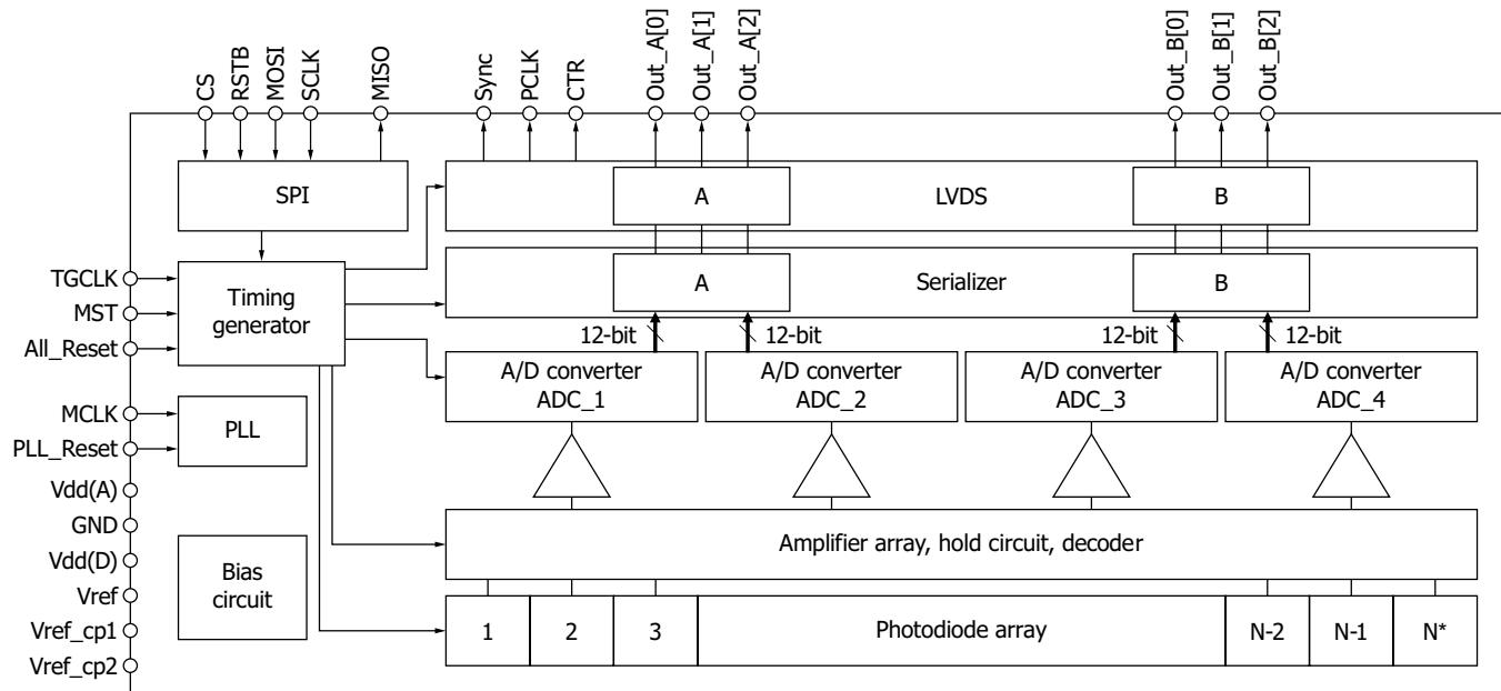
N=4096 (pixel size:  $7 \times 7 \mu\text{m}$ )
