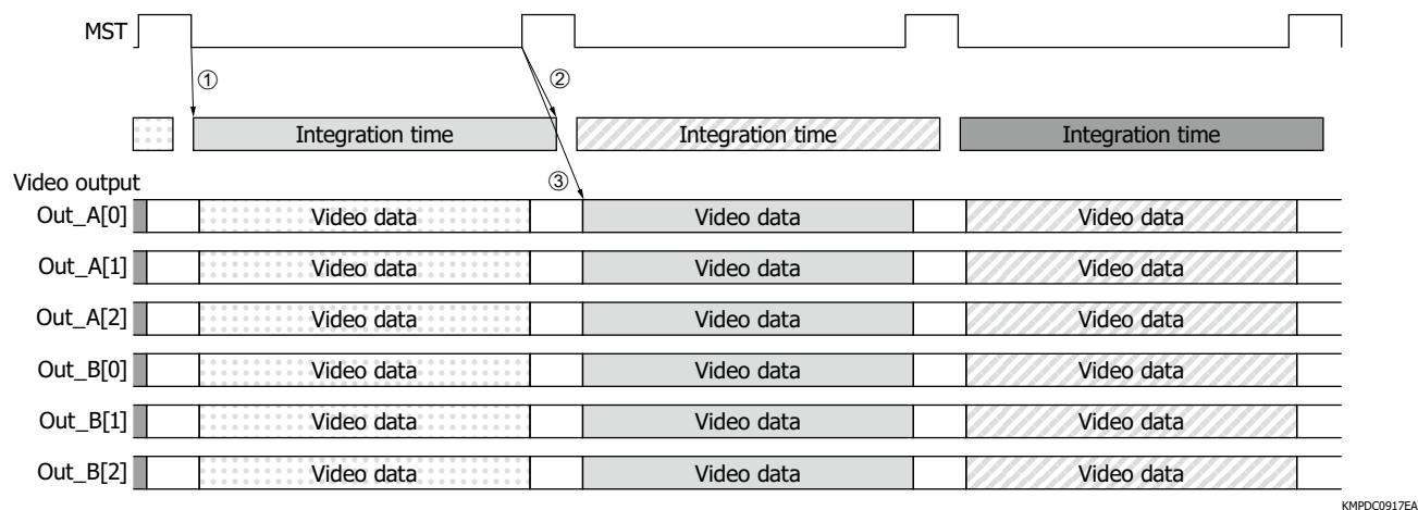
(1) The start of integration time is determined by the falling edge of the master start pulse.
