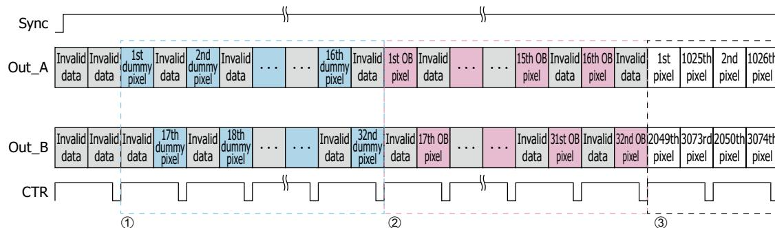
① From Out\_A, the 1st to 16th dummy pixels are read out sequentially.
