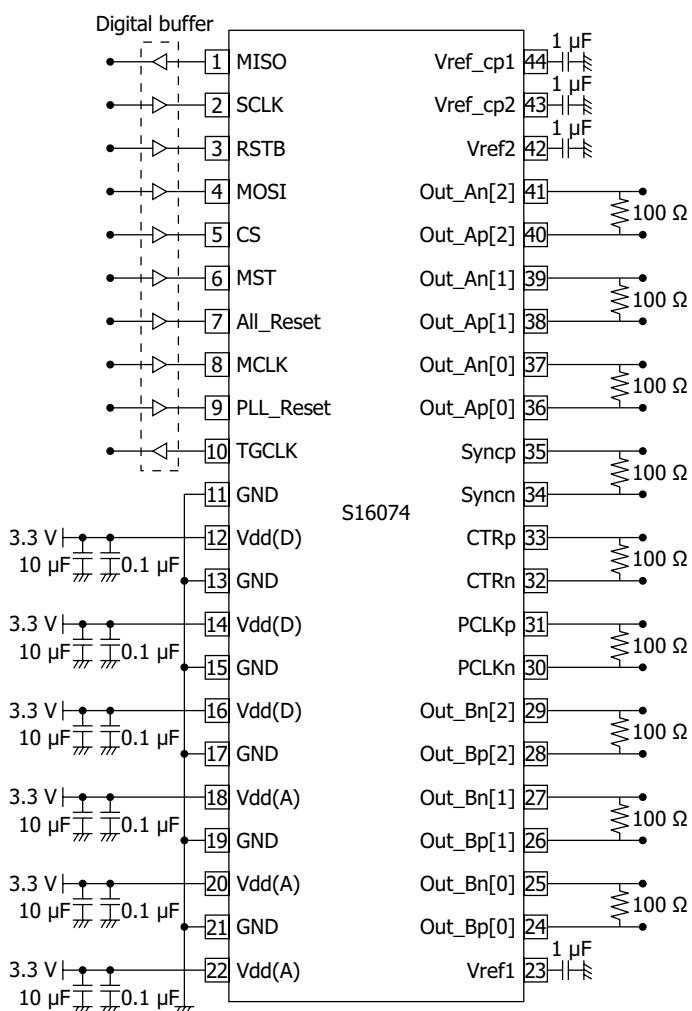
Note: Digital buffer is not necessary when MISO and TGCLK are not used.
