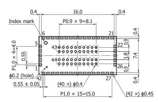
Tolerance unless otherwise noted  $\pm 0.25$ ,  $\pm 2.5^{\circ}$  Chip position accuracy with respect to package dimensions marked \* X, Y $\leq \pm 0.3$ ,  $\theta \leq \pm 2.5^{\circ}$  Au plating
