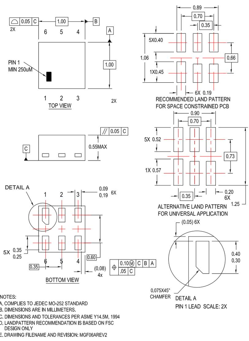
**Figure 10. 6-Lead, MicroPak2, 1x1mm Body, .35mm Pitch**
