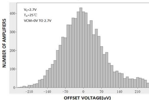
Input Offset Voltage Drift Distribution
