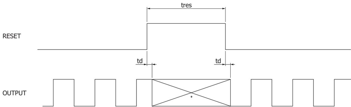
\* OUTPUT terminal is at High impedance during RESET period ("High" state).
