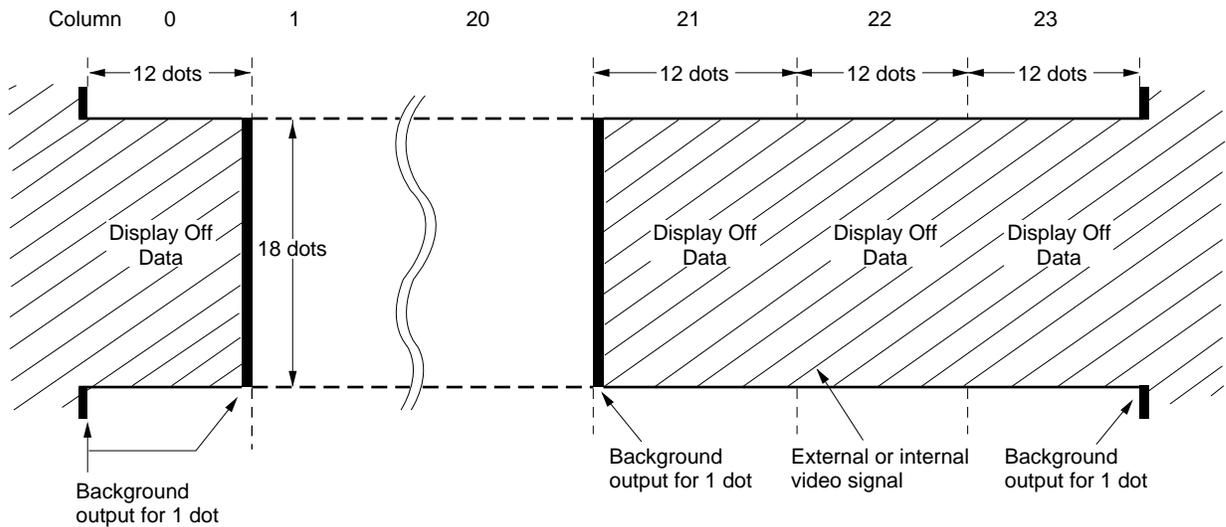
The background color is output on 1 dot on both the edges of Display Off Data when the Display Off Data is used.
