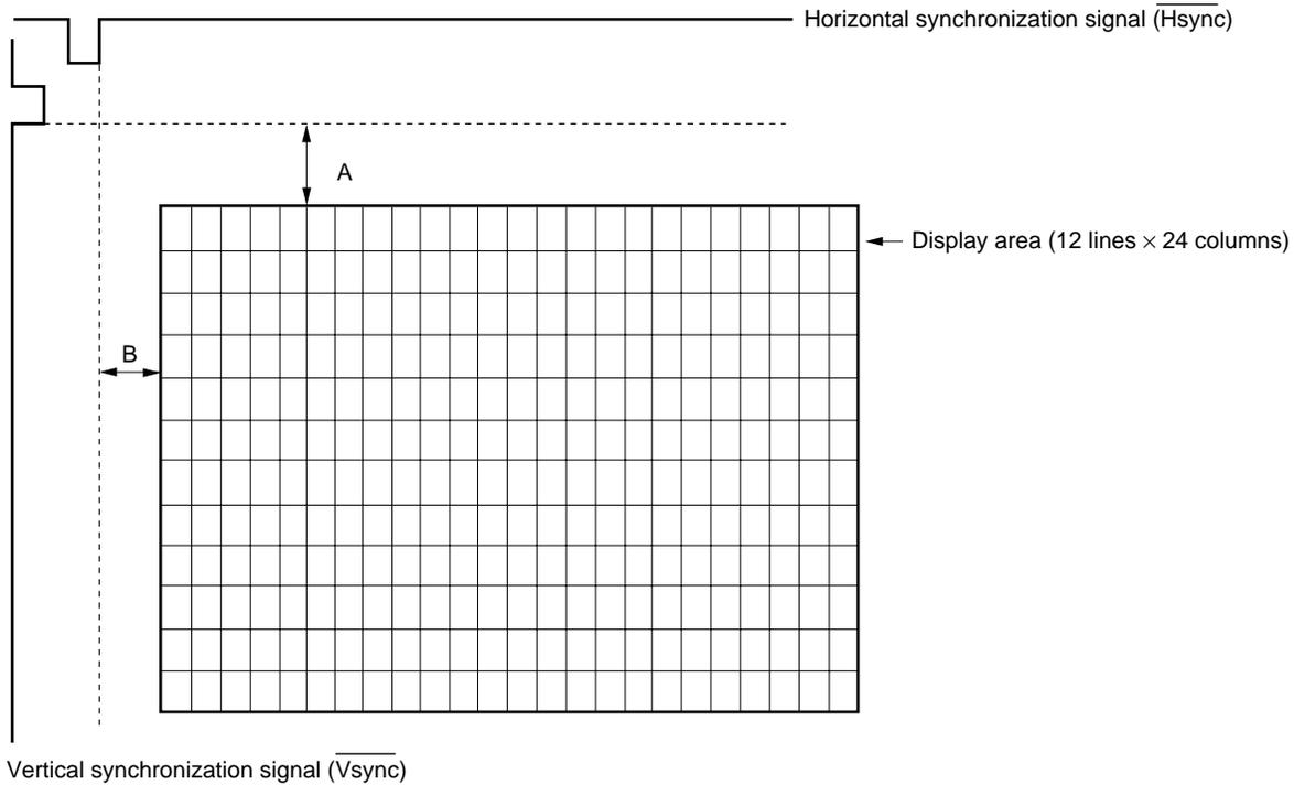
$$A: 9H \text{ (line)} \times (2^4V_4 + 2^3V_3 + 2^2V_2 + 2^1V_1 + 2^0V_0)$$
