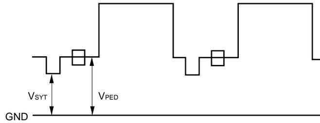
Match the level output from the VBSI pin in the external video signal mode with the level output from the same pin in the internal video signal mode.
