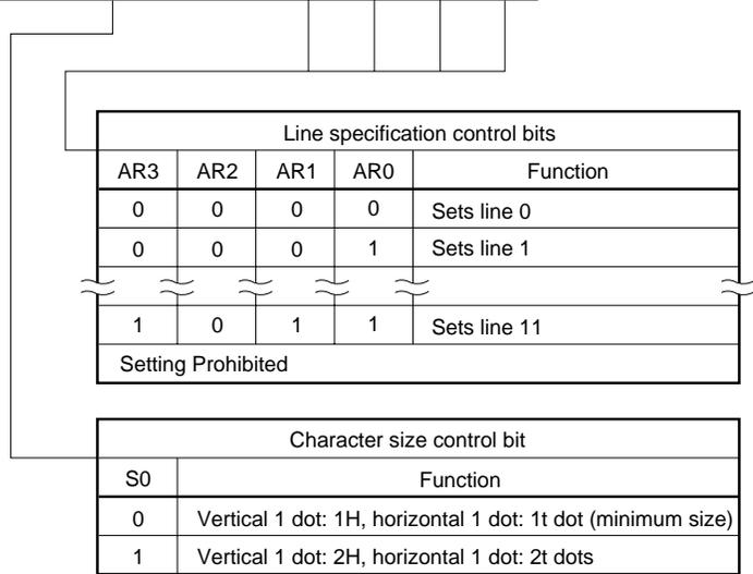
$$1t \text{ dot} = \frac{1}{f_{osc} \text{ (MHz)}} \mu\text{s}$$
