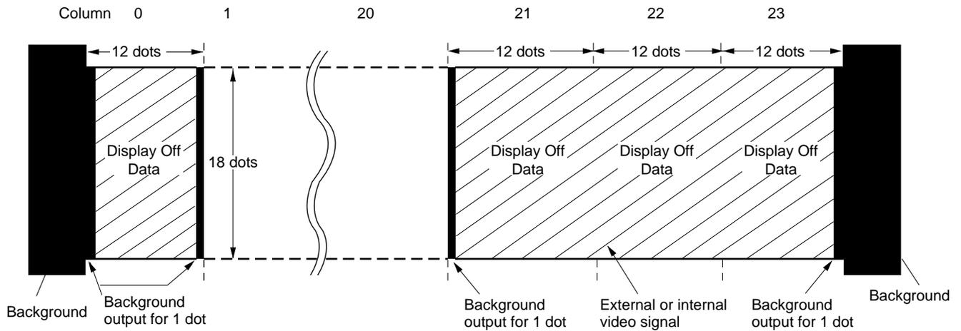
The background color is output on 1 dot on both the edges of Display Off Data when the Display Off Data is used.
