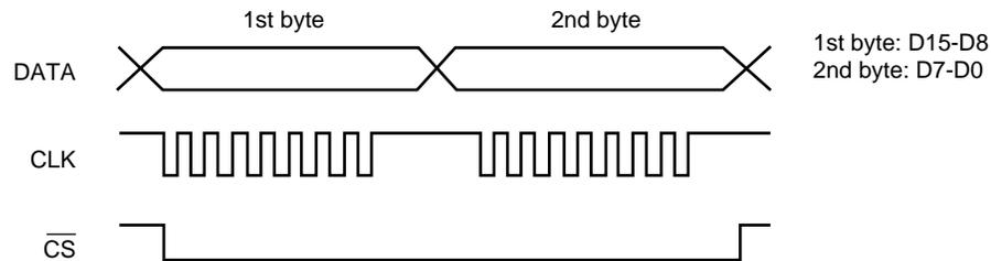
When transferring a 2-byte command, keep  $\overline{CS}$  low between the first byte and second byte.
