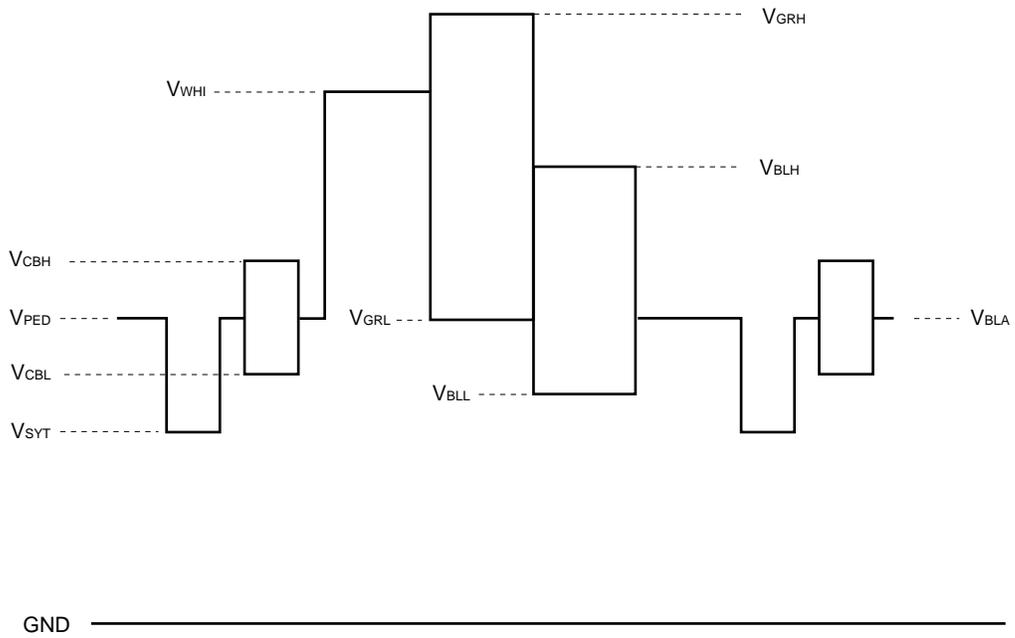
**Recommended Operation Timing (T<sub>A</sub> = -20 to +75 °C, V<sub>DD</sub> = 4.5 to 5.5 V)**
