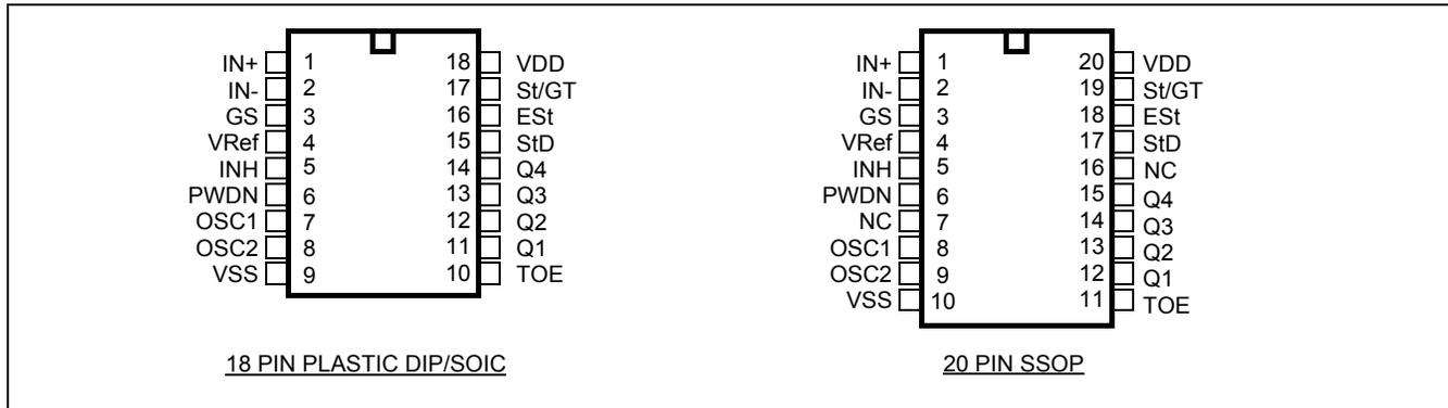
Figure 2 - Pin Connections
