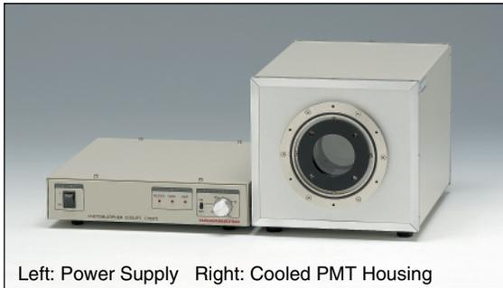
Left: Power Supply Right: Cooled PMT Housing
