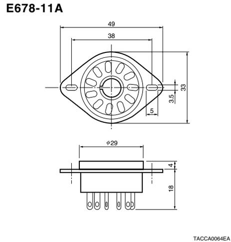
Figure 8: D Type Socket Assembly (Unit: mm) **Sold Separately**
