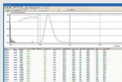
This screen shows the dependence of PL quantum yield on excitation wavelength. The excitation light through a motorized monochromator helps easily to measure wavelength dependence of the sample's PL quantum yield.
