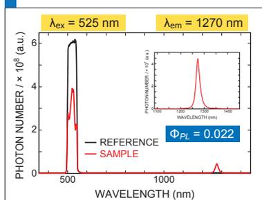
This is an example of the Photoluminescence quantum yield measurement of singlet oxygen using platinum (II) mesotetra (pentafluorophenyl) porphine (PtTFPP) solution as a sensitizer. We successfully expanded the wavelength region for the measurements to a 400 nm to 1650 nm range using a combination of BT-CCD and InGaAs line sensors.
