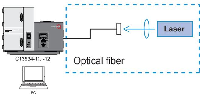
If you look for the option to use your own laser, please contact Hamamatsu, The laser should be guided to the system through the optical fiber, and then appropriate filters are required.
