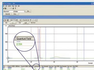
This is a basic screen for quantum yield measurements. The luminescence quantum yield is automatically calculated after measurement. Excitation and emission bands are defined by adjusting the cursors. The value of the quantum yield is displayed in the table below the spectrum next to emission intensities, peak wavelength, peak counts, and peak band (FWHM).
