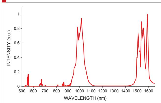
The measurement example of phosphor powder material (Y<sub>2</sub>O<sub>2</sub>S: Yb<sup>3+</sup>, Er<sup>3+</sup>) showing photoluminescence in NIR range. By excitation at 475 nm light, several emission bands were observed from Visible to NIR range (550 nm to 1,650 nm). Measurement setup: NIR PL measurement unit C13684-01, High power Xe lamp unit L13685-01, Filter unit A13687-01 and filter for excitation A13686-475.
