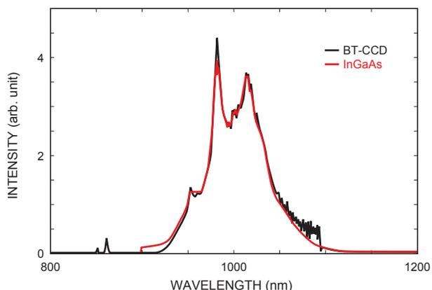
Figure. Emission spectra of Y<sub>2</sub>O<sub>2</sub>S: Yb,Er measured using BT-CCD and InGaAs linear image sensors.
