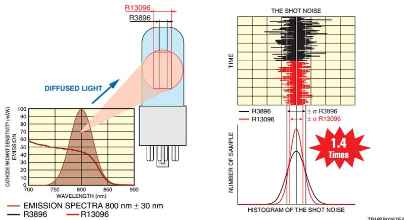
Figure 3: Typical Spectral Response
