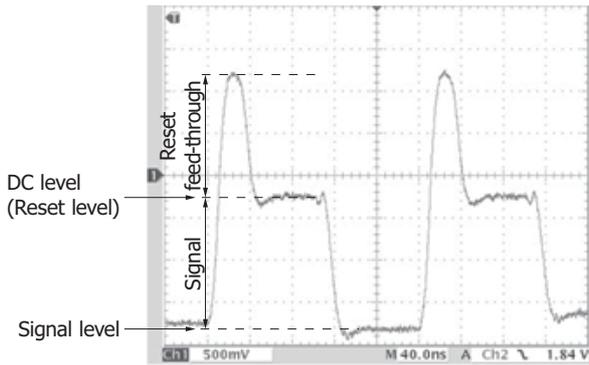
High-speed signal processing circuit example (using S11155/S11156-2048-02 and analog front-end IC)
