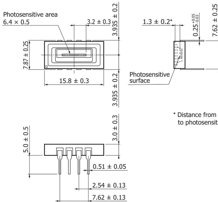
\* Distance from upper surface of window to photosensitive surface
