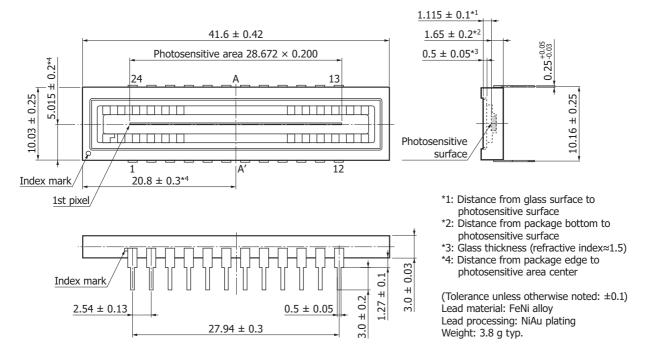
Note: This product is not hermetically sealed, and therefore moisture may penetrate into the package. Storing or using the product in a place with sudden temperature or humidity changes may cause condensation to form inside the package, so avoid such locations.
