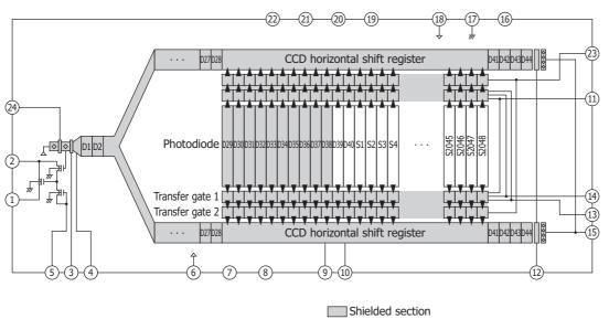
The signal charge photoelectrically converted in each pixel of the photosensitive area is separated and transferred vertically from the center of the photosensitive area.
