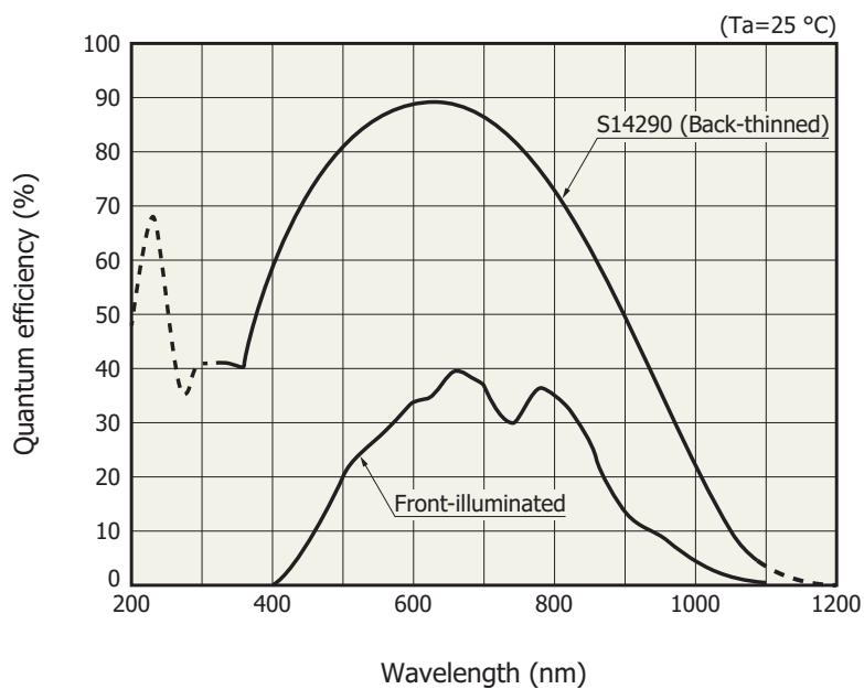
\*17: Spectral response with borosilicate glass is decreased according to the spectral transmittance characteristics of window material.
