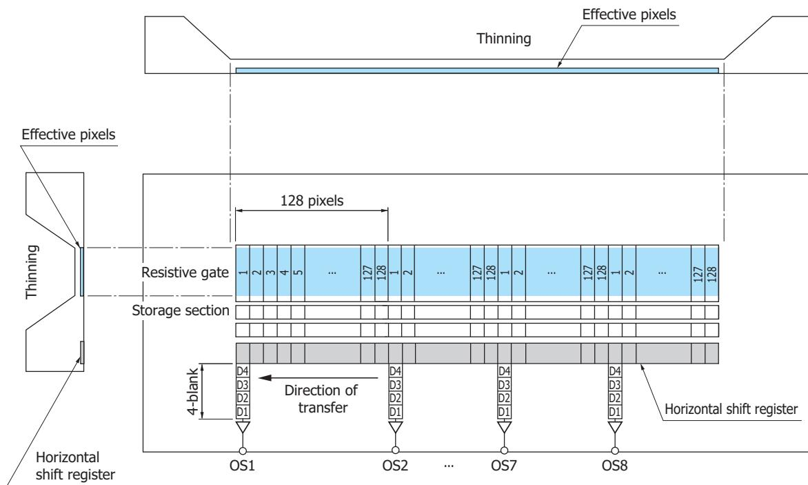
Note: When viewed from the direction of the incident light, the horizontal shift register is covered with a thick silicon layer (dead layer). However, long-wavelength light passes through the silicon dead layer and may possibly be detected by the horizontal shift register. To prevent this, provide light shield on that area as needed.
