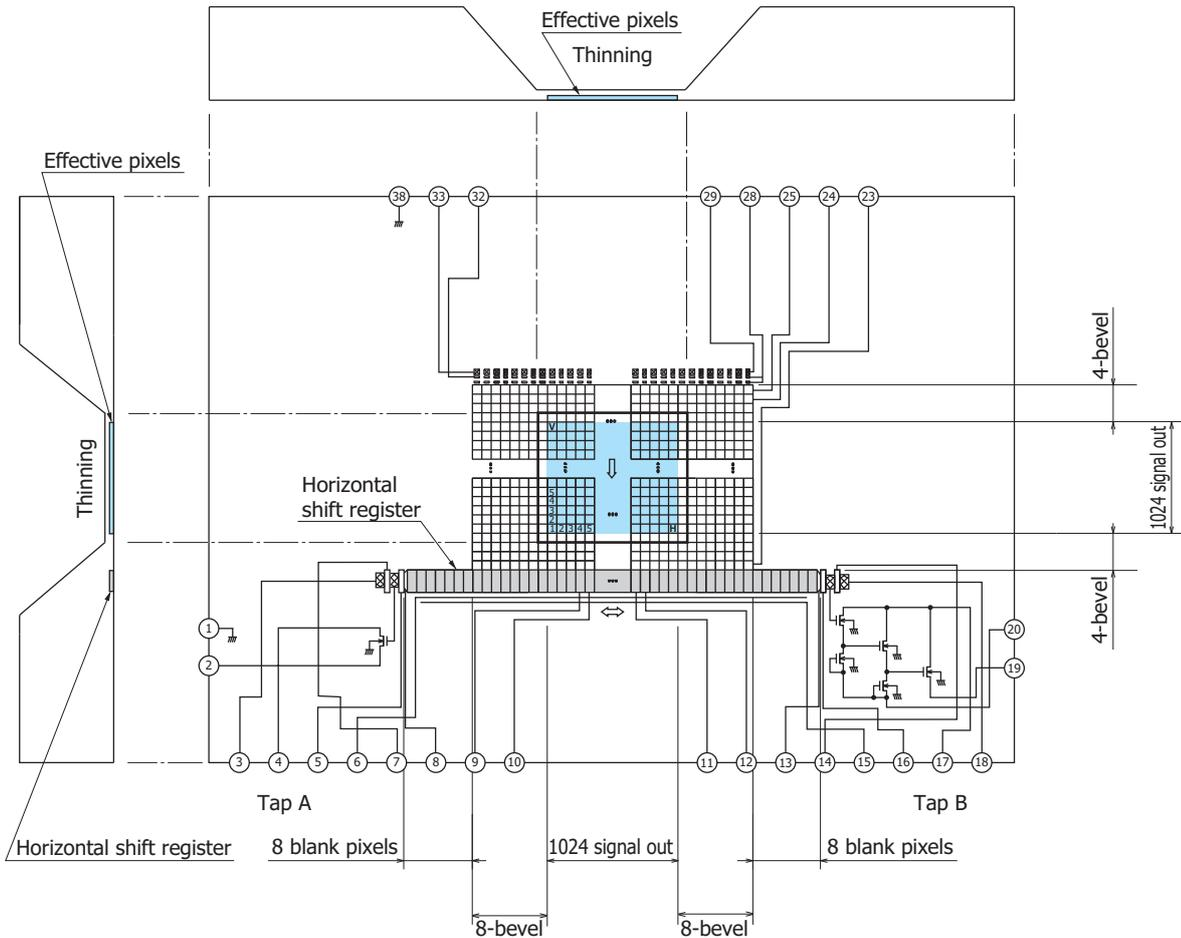
Note: When viewed from the direction of the incident light, the horizontal shift register is covered with a thick silicon layer (dead layer). However, long-wavelength light passes through the silicon dead layer and may possibly be detected by the horizontal shift register. To prevent this, provide light shield on that area as needed.
