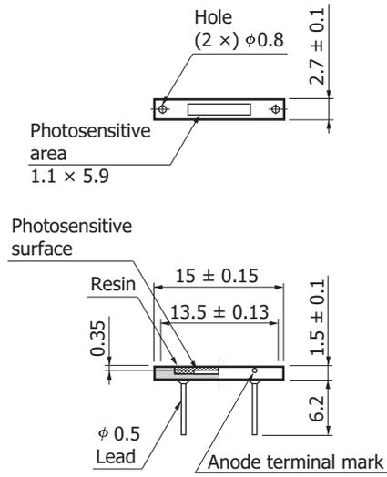
The resin potting may extend a maximum of 0.1 mm above the upper surface of the package.
