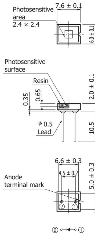
The resin potting may extend a maximum of 0.1 mm above the upper surface of the package.
